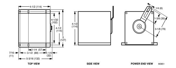
Fig. 2—Limits of crank arm rotation.
