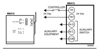
Fig. 20—M8405 Damper Actuator three-position wiring connections.
