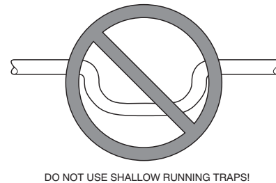
Fig. 19 - Insufficient Condensate Trap
