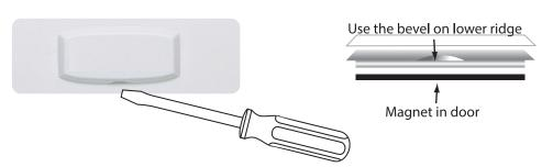
Gently slide a screwdriver into the bottom edge of the badge. Gently turn the screwdriver counter clockwise. The badge is held on by a magnet in the well of the battery door. The badge should pry off easily. Do not use force.
